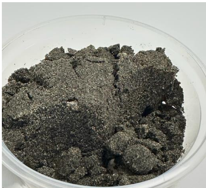
Figure 14: Sample 3 (depth 31,35-32,32m) with a sulfate concentration of 2130,1 mg/kg and a chloride concentration of 2800,0 mg/kg. It has a chloride concentration of 4059,9mg/kg.
