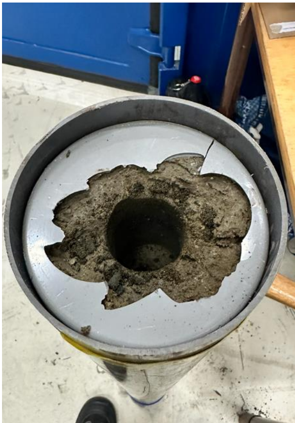
Figure 10: Sample 42 was cracked open with a hammer, sampled with a borer, and then later sealed with parafilm and duct tape.
