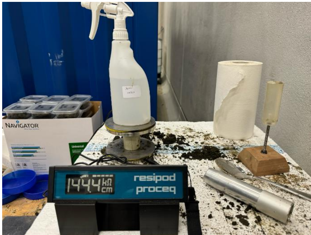
Figure 9: Make-shift resistivity cell at COVRA premises. (Image by author)
