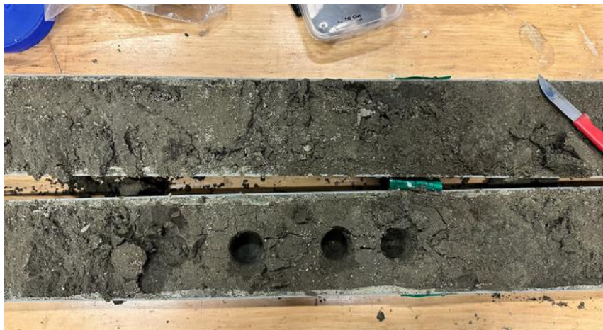
Figure 5: Soil was taken from sample 58 using the soil borer.
