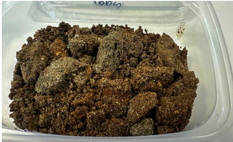
Figure 14: Sample 3 (depth 31,35-32,32m) with a sulfate concentration of 2130,1 mg/kg and a chloride concentration of 2800,0 mg/kg. It has a chloride concentration of 4059,9mg/kg.
