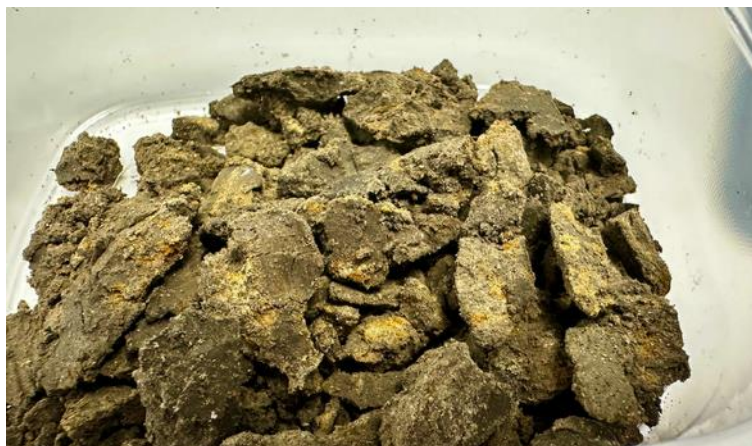
Figure 11: Sample 43 (depth 68,89m-69,89m) showing red-brown patches of iron. It has the highest sulfate level of all the samples (19388,9 mg/kg). It has a chloride concentration of 3644,2mg/kg.
