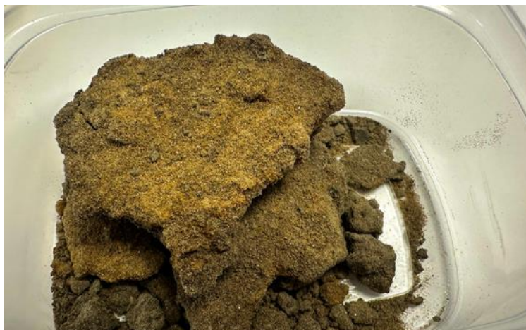
Figure 12: Sample 46 (depth 72,45-73,44m) showing patches of iron. Sulfate concentration of 11061,1 mg/kg. It has a chloride concentration of 3446,6mg/kg.
