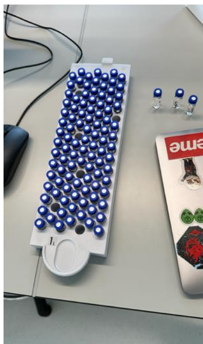
Figure 8: IC vials in chromatographer tray before running the chromatogram.
