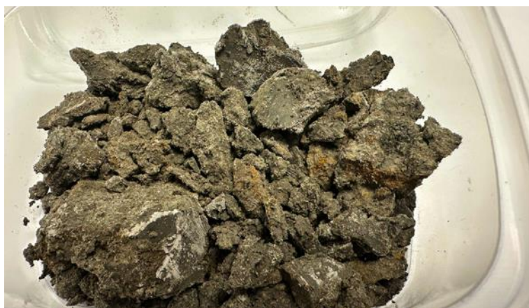
Figure 12: Sample 46 (depth 72,45-73,44m) showing patches of iron. Sulfate concentration of 11061,1 mg/kg. It has a chloride concentration of 3446,6mg/kg.
