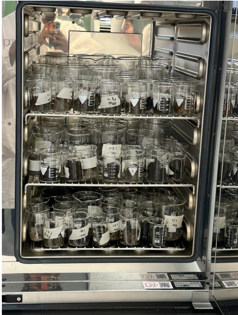
Figure 6: All the weighed samples in the oven before drying
