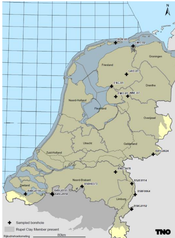
Figure 1: Visual representation of the extent of Boom Clay Member throughout nearly all of the onshore Netherlands as well as northern Belgium and specifically in the Campine Basin. Produced by TNO and published in a desk –study report studying the geohydrological properties of Boom Clay specifically in the Dutch subsurface, hence the borehole locations denoted as crosses (G.-J. Vis & J.M. Verweij, 2014).
