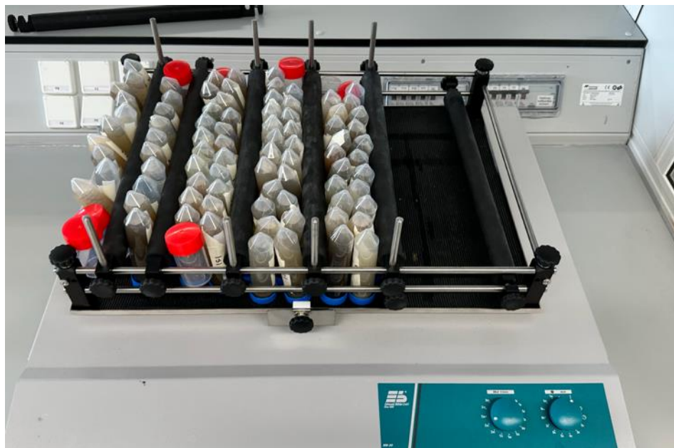
Figure 7: Samples placed in shaker prior to centrifugation
