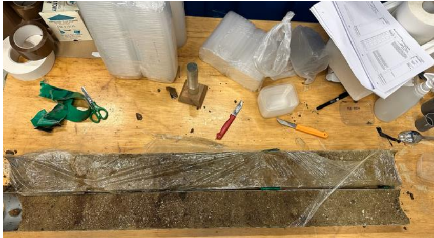
Figure 4: Sample 2 split open. The soil borer and plastic containers can be seen placed above the sample.
