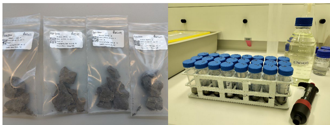
Figure 2.1. Left: bags with subsamples of shoe samples from DAPGEO-02 as received from TU Delft. Right: Centrifuge tubes with samples during the sequential extraction.
