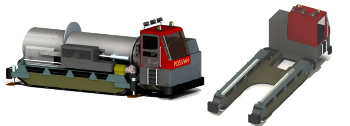
Figure 6-1: Left: Canister installation vehicle, right: canister installation vehicle's chassis in a view obliquely from the rear. The radiation shield and the canister are missing from the picture. Both pictures based on (Wendelin & Suikki 2008)
