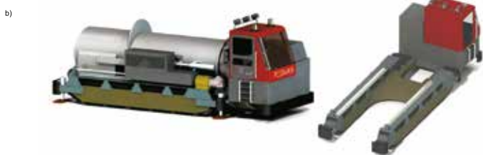
Figure 4.5a) The emplacement of a HLW package in a disposal tunnel. After the emplacement of the HLW package, part of the tunnel will be backfilled. For retrieval, the process is essentially reversed. The drawing is at scale, except for the centre – centre distance between the packages: the distance shown on the figure is smaller than the actual distance between two HLW packages. b) The emplacement vehicle developed by Posiva Oy (Finland). While this is not developed for a disposal concept in which the HLW package will be transported vertically, it has the same functionality required for our reference GDF design.
