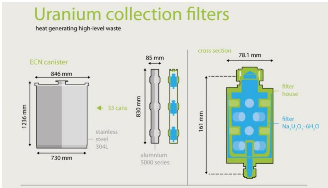
Figure 6: Schematic showing Uranium Collection Filters and ECN container (from Verhoef et al., 2016)
