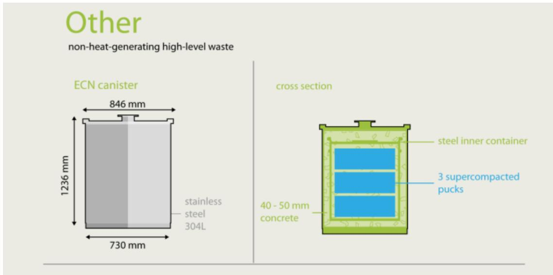
**Figure 7: ECN container for 'other' non-heat generating waste (from Verhoef et al., 2016)**
