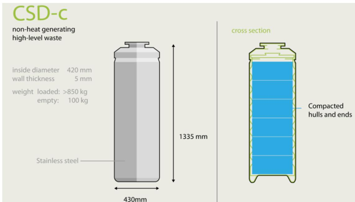
**Figure 2: Areva/Orano Colis Standard de Déchets (CSD) waste container used for vitrified waste and compacted hulls and ends (from Verhoef et al., 2016)**
