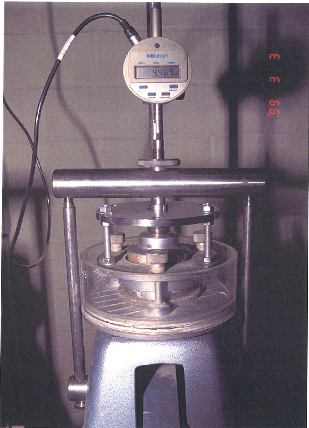
Figure 4.9 Fixed-ring cell adapted for high pressures.
