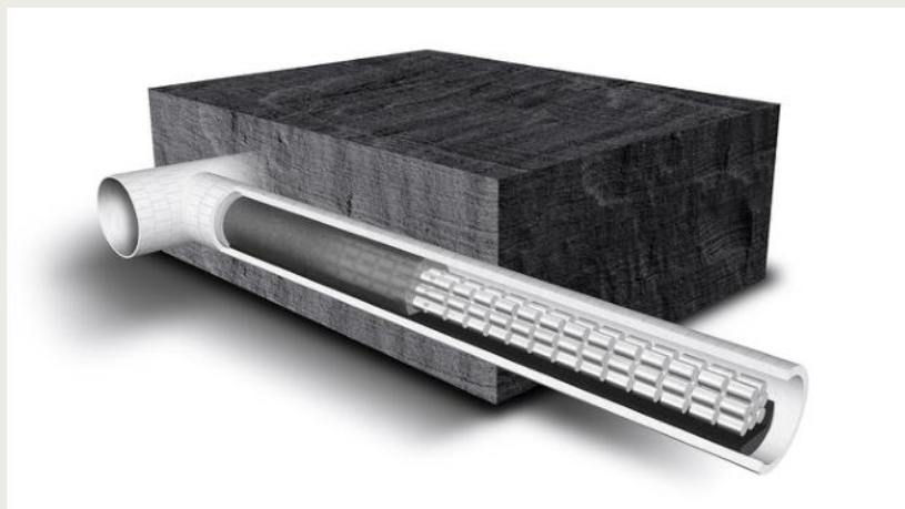
Figure 3 Disposal of the LILW containers in the LILW disposal gallery
