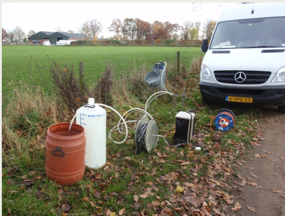
Figure 2-2. Sampling of a deep screen using a submersible pump
