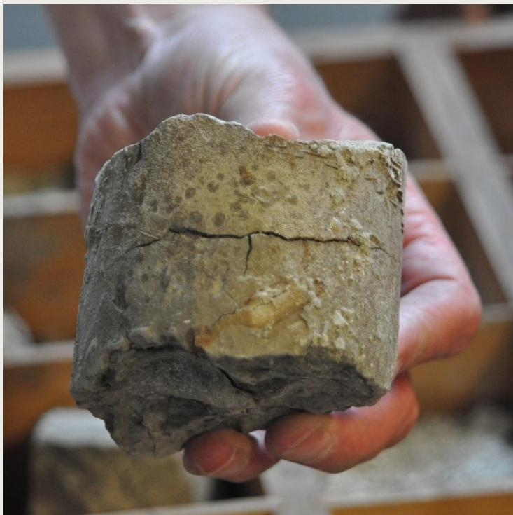
Figure 2. A piece of Boom Clay from several hundreds of meters depth. The circular spots could be secondary gypsum after pyrite oxidation.
