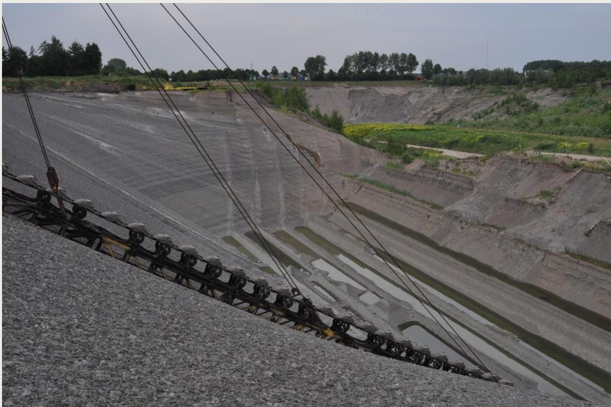
Figure 18. The Boom Clay as it appears in a quarry near Antwerp (Belgium) showing its horizontally layered structure.
