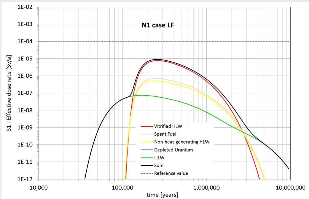
Figure 3-14 Contribution of the various disposal sections to the effective dose rate (S1). Calculation case N1-LF. PA model version 9.3.
