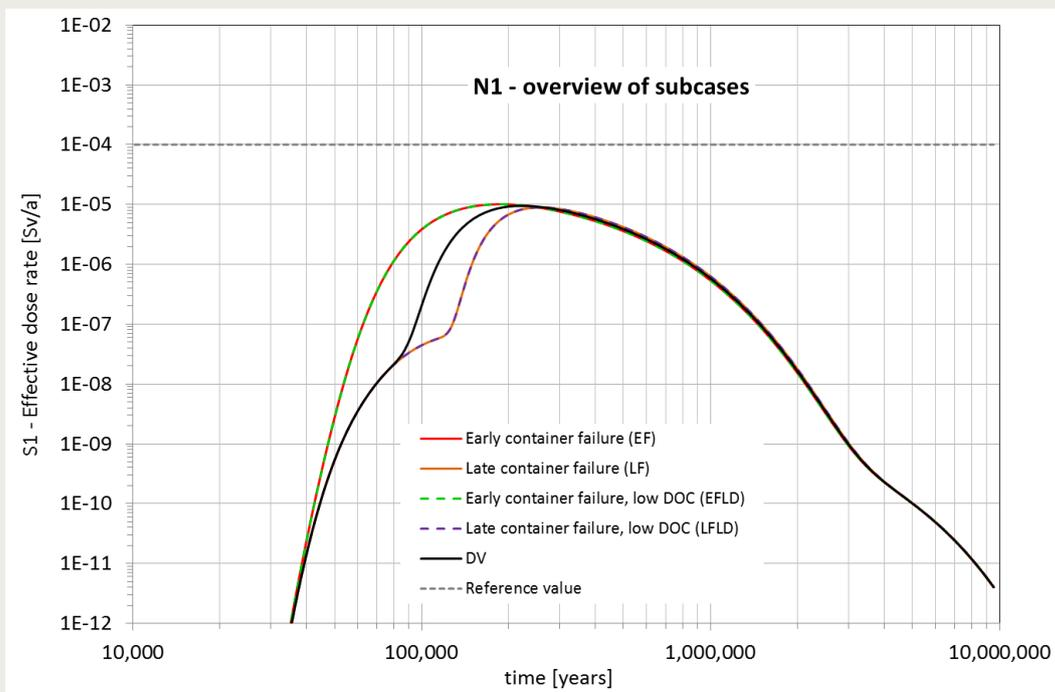
Figure 4-1 Effective dose rate (S1) - Calculation cases DV, EF, LF, EFLD, and LFLD
