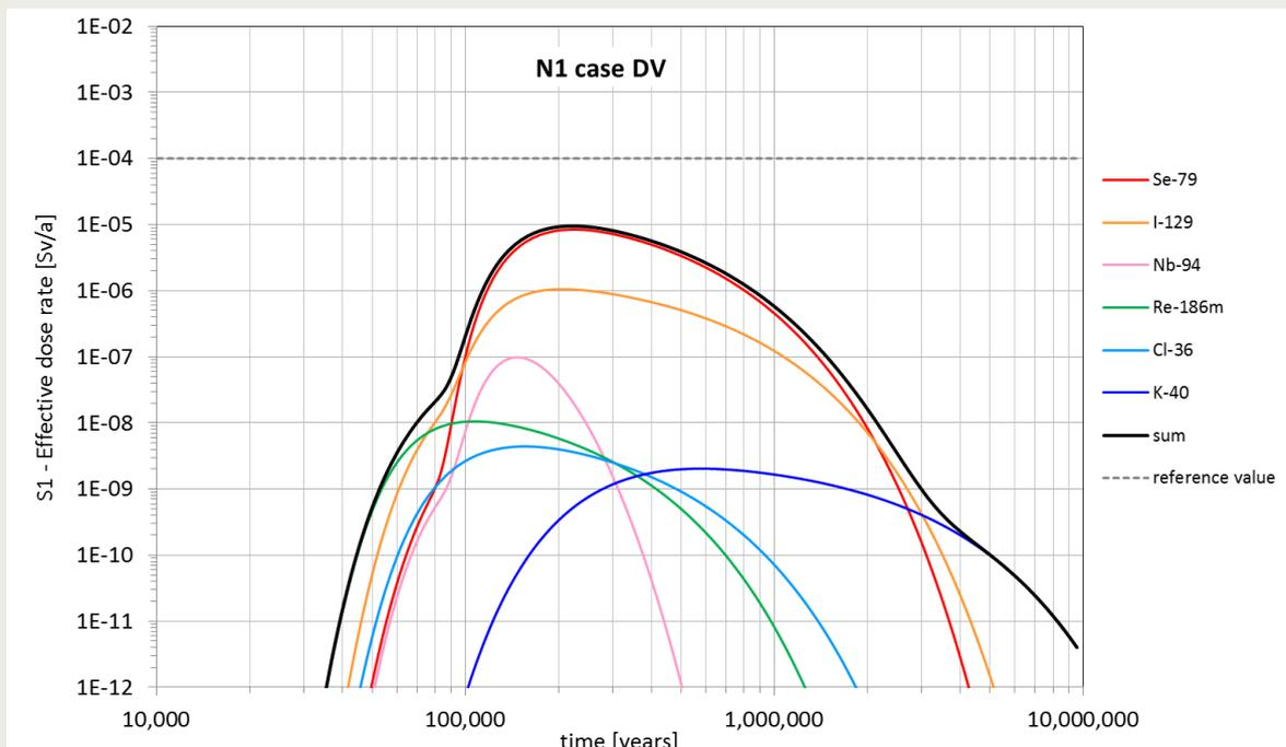
Figure 3-1 Effective dose rate (S1). Calculation case N1-DV. PA model version 9.3.
