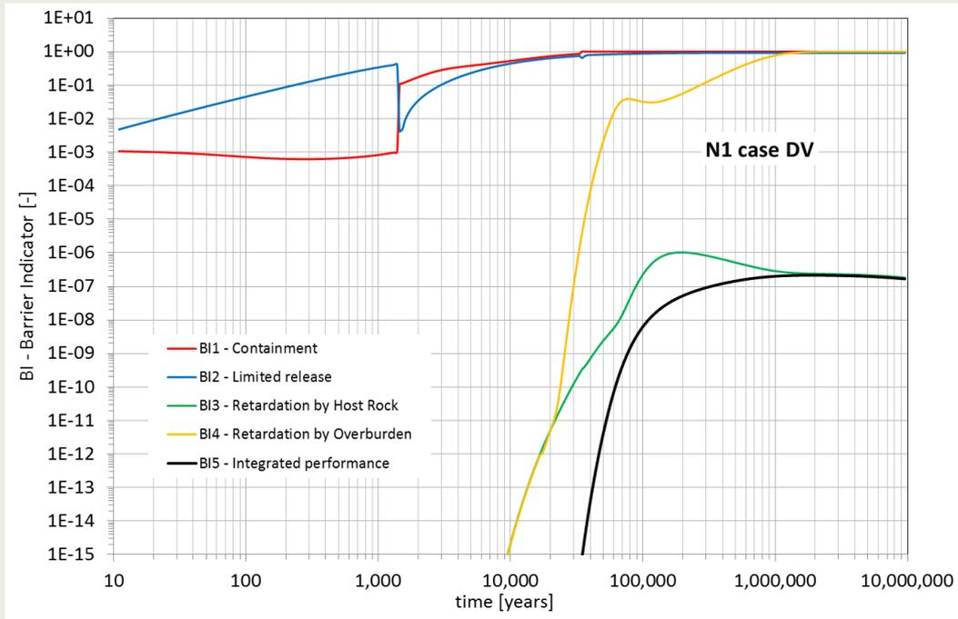
Figure 3-5 Performance of the integrated repository system (BI5). Calculation case N1-DV. PA model version 9.3.
