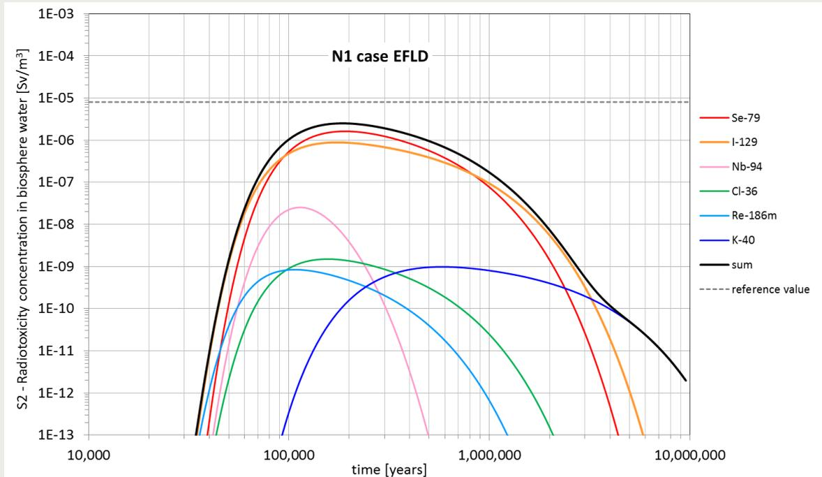
Figure 3-22 Radiotoxicity concentration in biosphere water (S2). Calculation case N1-EFLD. PA model version 9.3
