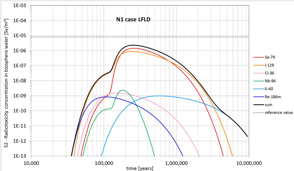
Figure 3-28 Radiotoxicity concentration in biosphere water (S2). Calculation case N1-LFLD. PA model version 9.3.
