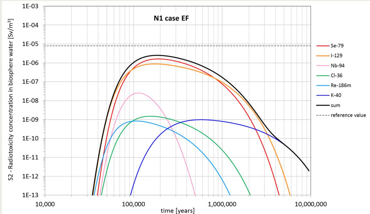
Figure 3-10 Radiotoxicity concentration in biosphere water (S2). Calculation case N1-EF. PA model version 9.3.
