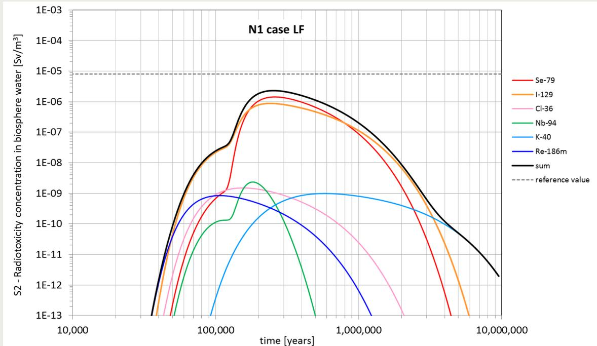
Figure 3-16 Radiotoxicity concentration in biosphere water (S2). Calculation case N1-LF. PA model version 9.3.
