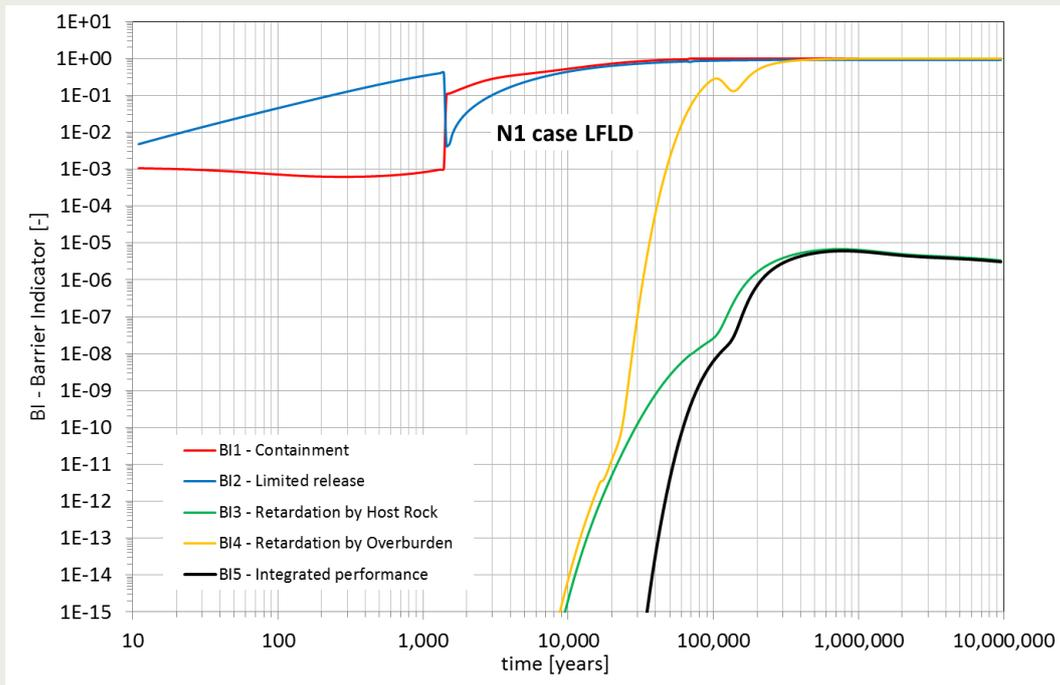
Figure 3-29 Performance of the integrated repository system (BI5). Calculation case N1-LFLD. PA model version 9.3.
