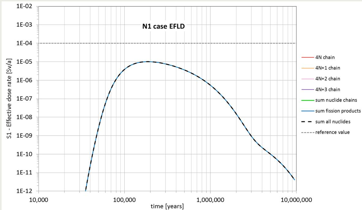
Figure 3-21 Contribution of the natural nuclide decay chains to the effective dose rate (S1). Calculation case N1-EFLD. PA model version 9.3.
