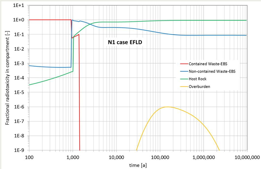
Figure 3-24 Fractional radiotoxicity of the different compartments of the repository system. Calculation case N1-EFLD. PA model version 9.3.
