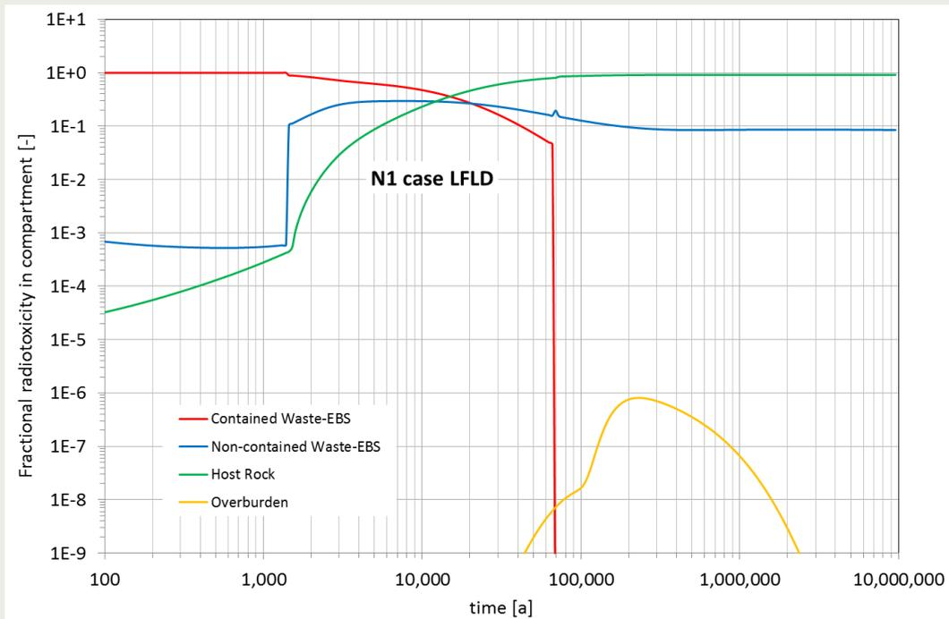
Figure 3-30 Fractional radiotoxicity of the different compartments of the repository system. Calculation case N1-LFLD. PA model version 9.3.
