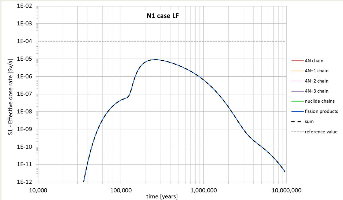
Figure 3-15 Contribution of the natural nuclide decay chains to the effective dose rate (S1). Calculation case N1-LF. PA model version 9.3.
