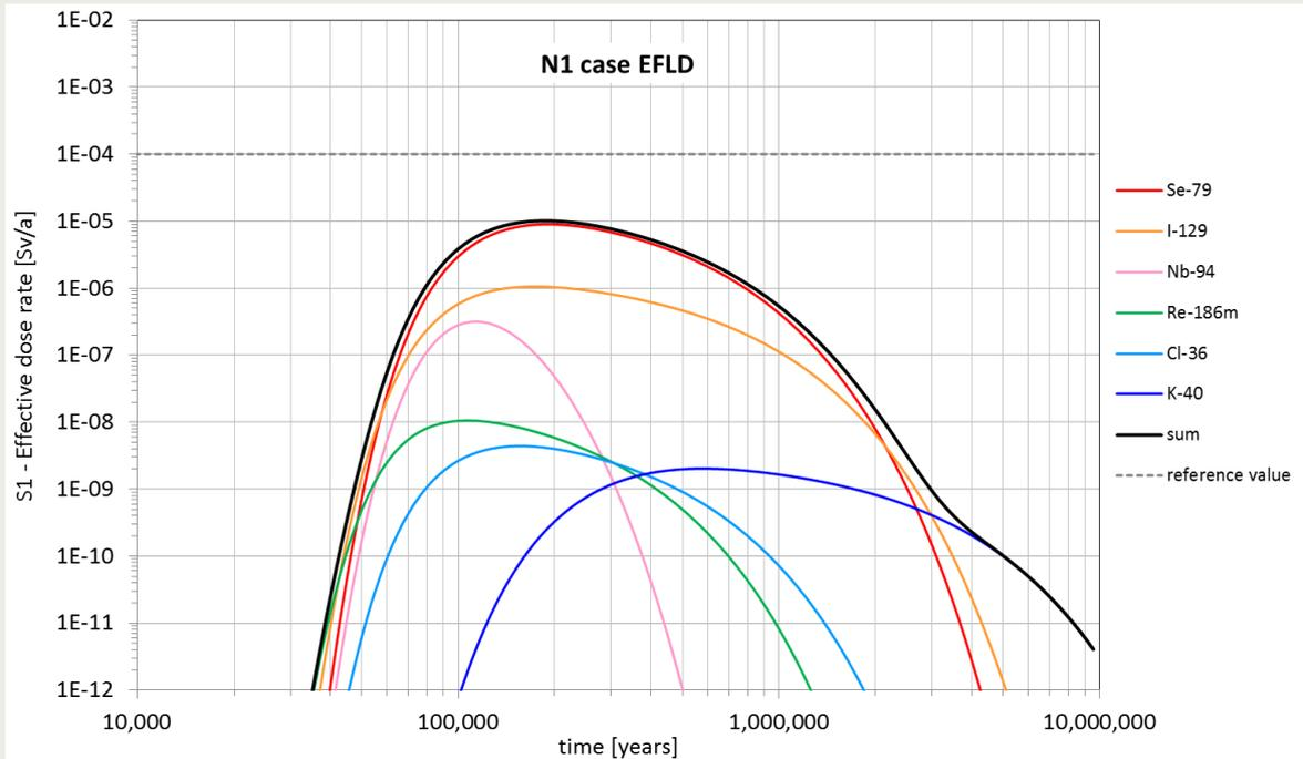
Figure 3-19 Effective dose rate (S1). Calculation case N1-EFLD. PA model version 9.3.
