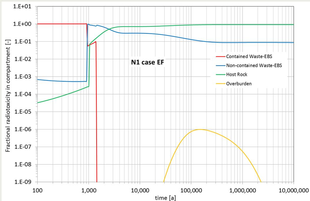
Figure 3-12 Fractional radiotoxicity of the different compartments of the repository system. Calculation case N1-EF. PA model version 9.3.
