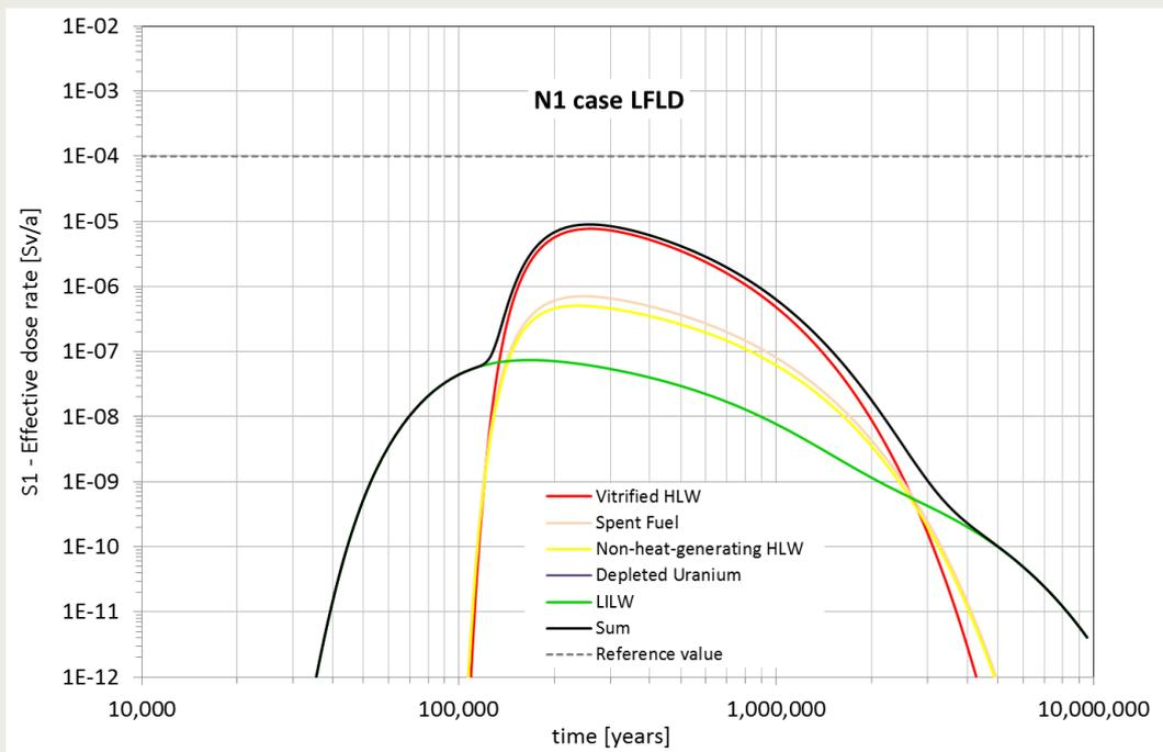
Figure 3-26 Contribution of the various disposal sections to the effective dose rate (S1). Calculation case N1-LFLD. PA model version 9.3.
