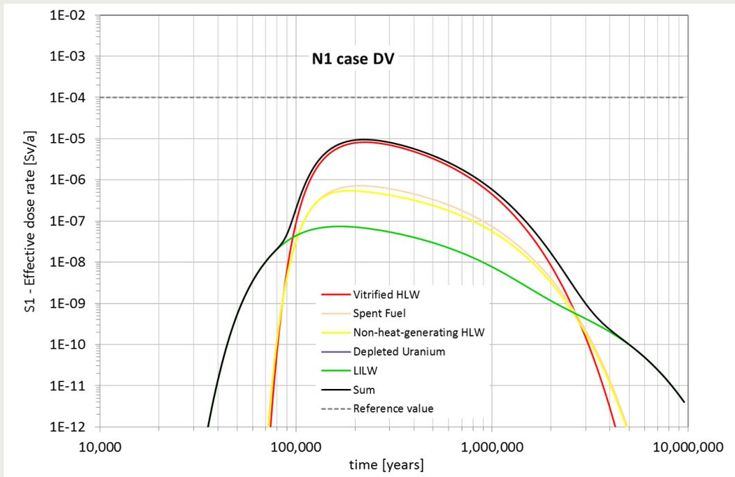
Figure 3-2 Contribution of the various disposal sections to the effective dose rate (S1). Calculation case N1-DV. PA model version 9.3.
