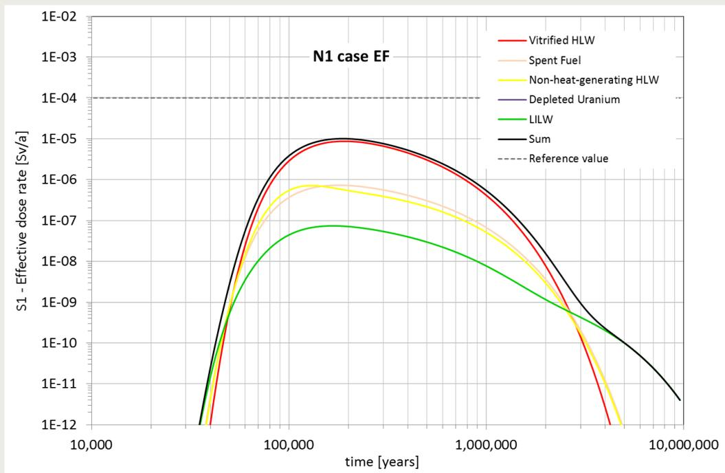
Figure 3-8 Contribution of the various disposal sections to the effective dose rate (S1). Calculation case N1-EF. PA model version 9.3.
