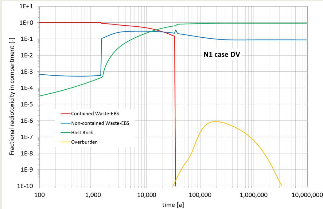
Figure 3-6 Fractional radiotoxicity of the different compartments of the repository system. Calculation case N1-DV. PA model version 9.3.
