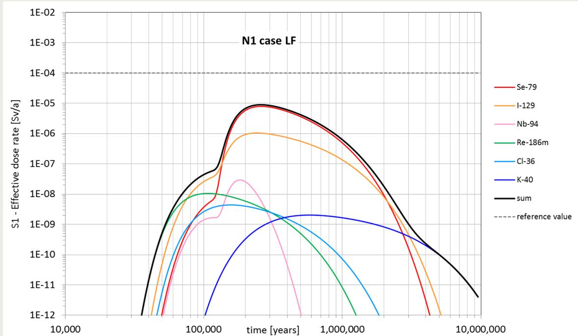
Figure 3-13 Effective dose rate (S1). Calculation case N1-LF. PA model version 9.3.
