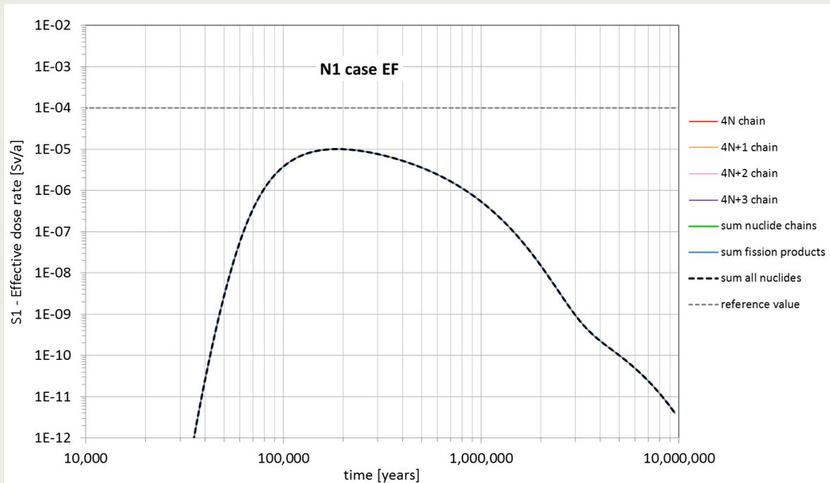
Figure 3-9 Contribution of the natural nuclide decay chains to the effective dose rate (S1). Calculation case N1-EF. PA model version 9.3.
