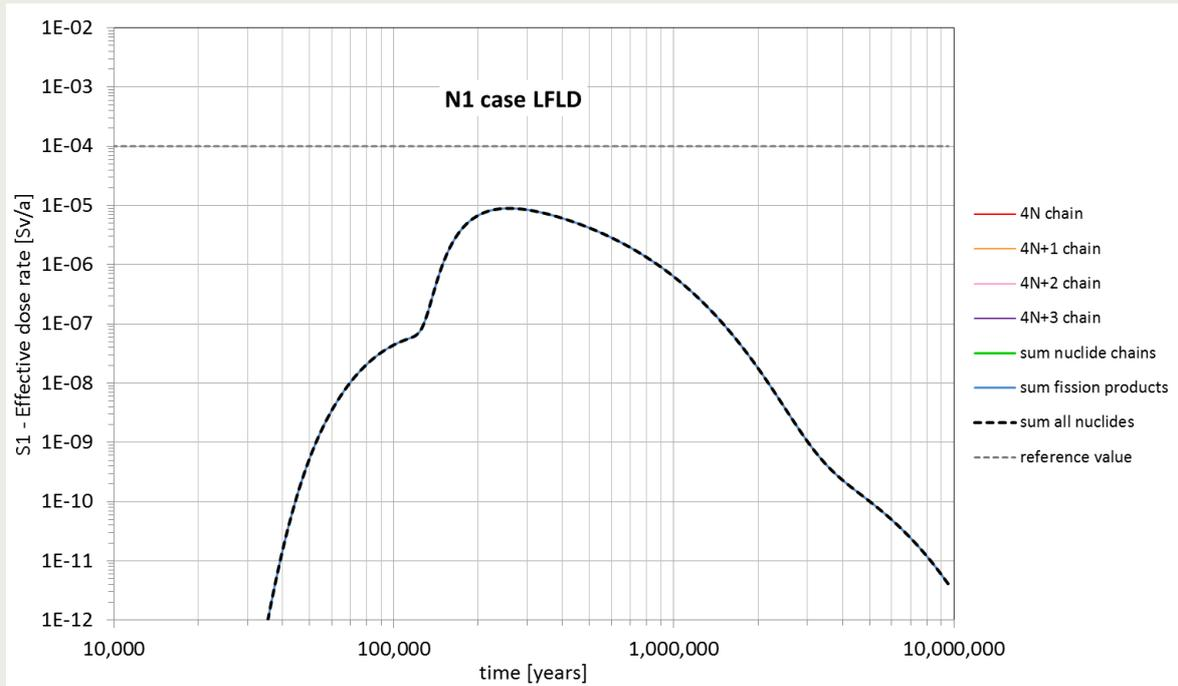
Figure 3-27 Contribution of the natural nuclide decay chains to the effective dose rate (S1). Calculation case N1-LFLD. PA model version 9.3.
