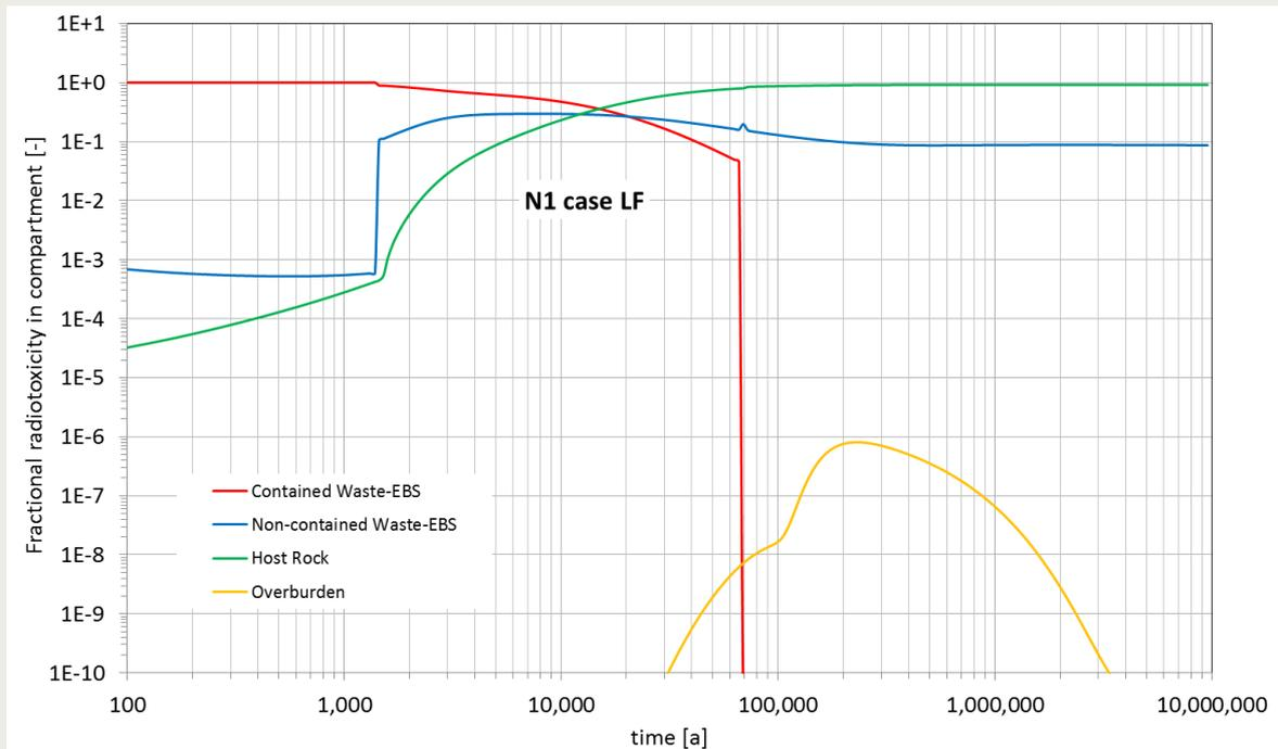
Figure 3-18 Fractional radiotoxicity of the different compartments of the repository system. Calculation case N1-LF. PA model version 9.3.
