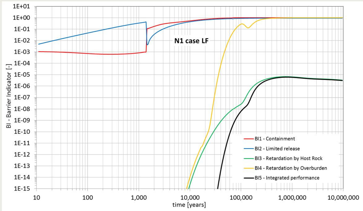
Figure 3-17 Performance of the integrated repository system (BI5). Calculation case N1-LF. PA model version 9.3.
