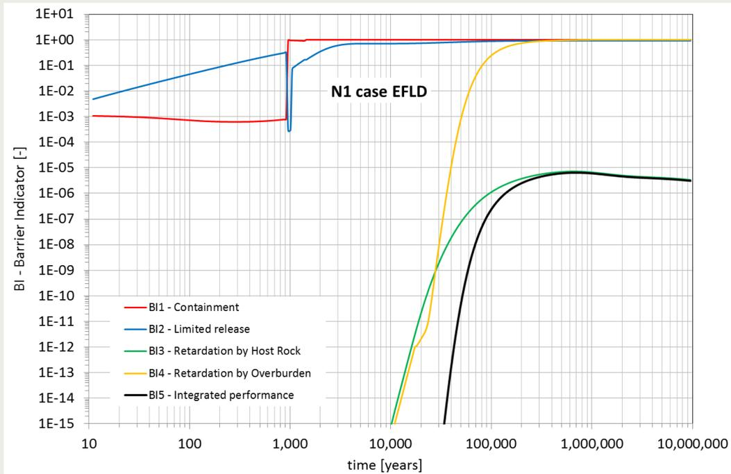
Figure 3-23 Performance of the integrated repository system (BI5). Calculation case N1-EFLD. PA model version 9.3.
