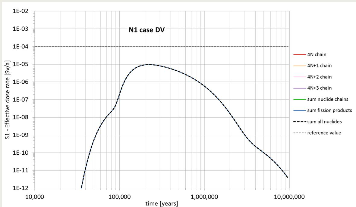
Figure 3-3 Contribution of the natural nuclide decay chains to the effective dose rate (S1). Calculation case N1-DV. PA model version 9.3.
