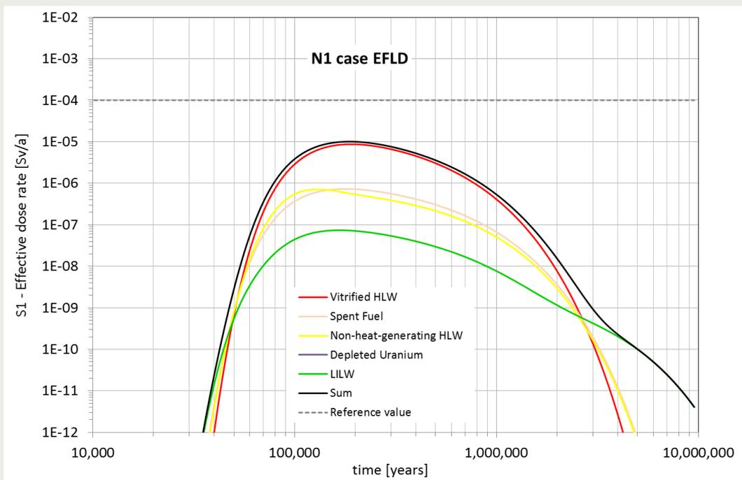
Figure 3-20 Contribution of the various disposal sections to the effective dose rate (S1). Calculation case N1-EFLD. PA model version 9.3.
