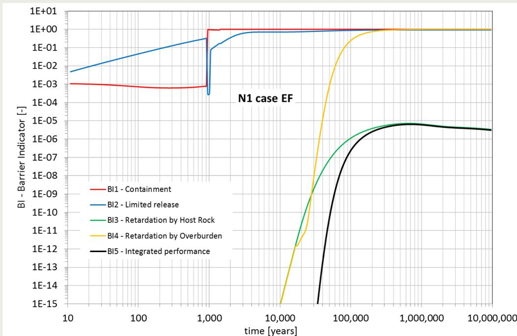
Figure 3-11 Performance of the integrated repository system (BI5). Calculation case N1-EF. PA model version 9.3.
