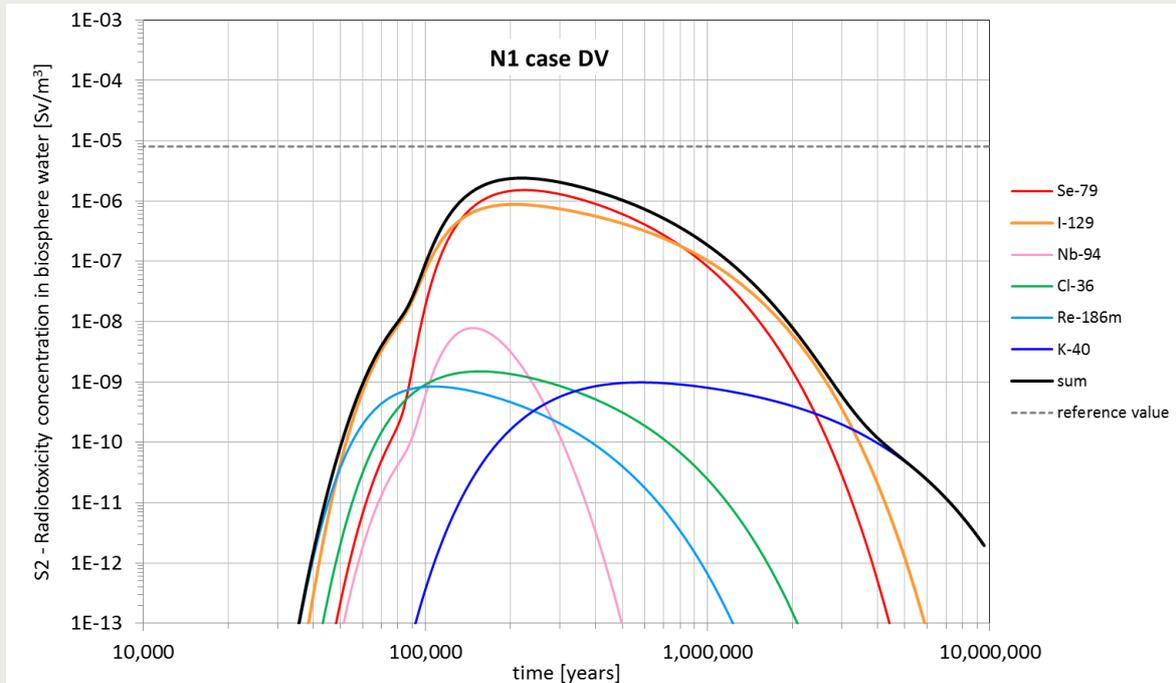
Figure 3-4 Radiotoxicity concentration in biosphere water (S2). Calculation case N1-DV. PA model version 9.3.
