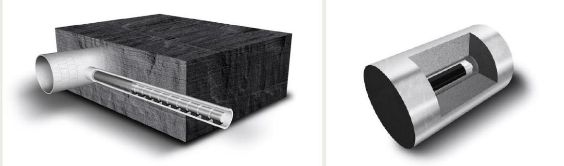
Figure 3-1: Artist impression of the waste compartments and the OPERA supercontainer [Verhoef, 2014a].
