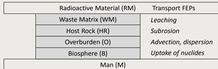
**Figure 6-13 Multi Barrier System for the subrosion scenario**
