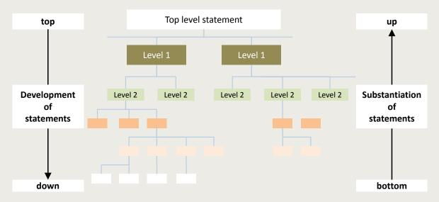
Figure 3-1 The top-down development of the structured set of safety statements and the bottom-up assessment of the level of support for these statements.
