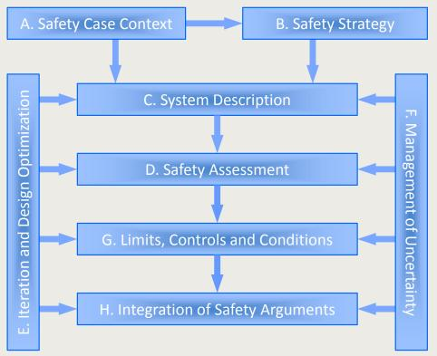
Figure 2-2 Components of a Safety Case
