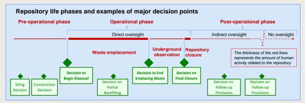
Figure 2-1 Phases of a disposal facility.
