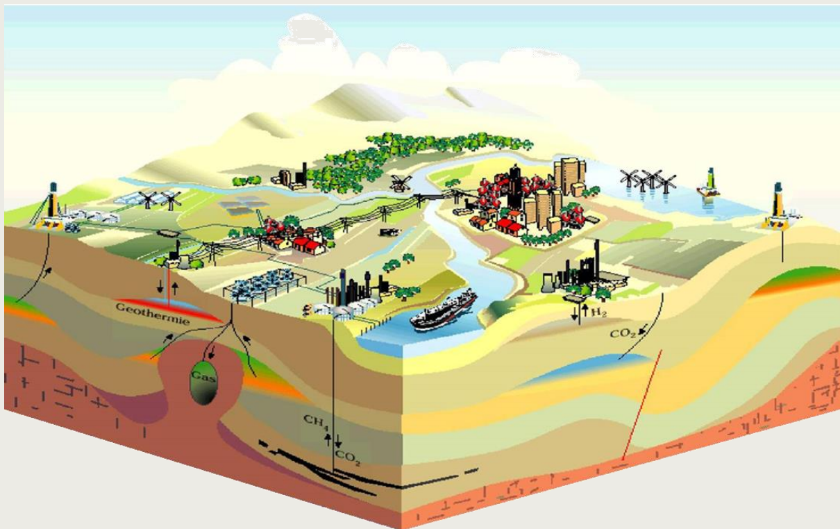
Figure C.1-1: Artist impression of infrastructure at the earth's surface and subsurface for capture, transport and storage of CO 2 (courtesy TNO, 2015)
