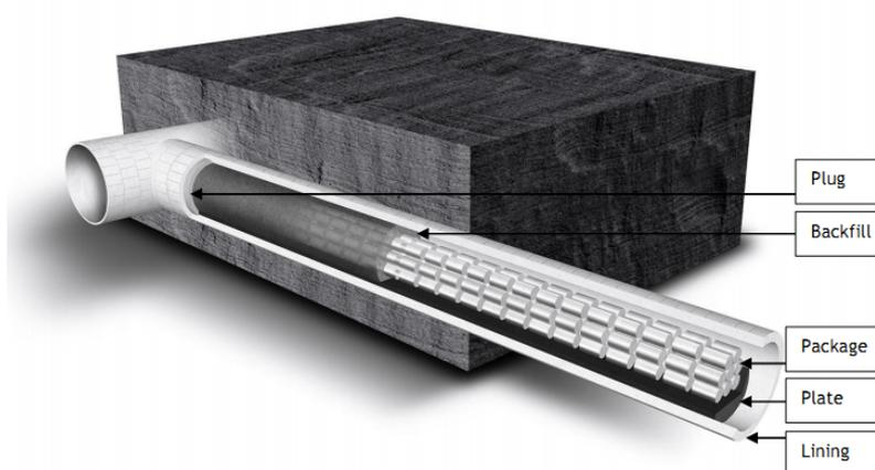
Figure 3: Scheme of the LILW section with 1,000 L containers [Verhoef 2014]
