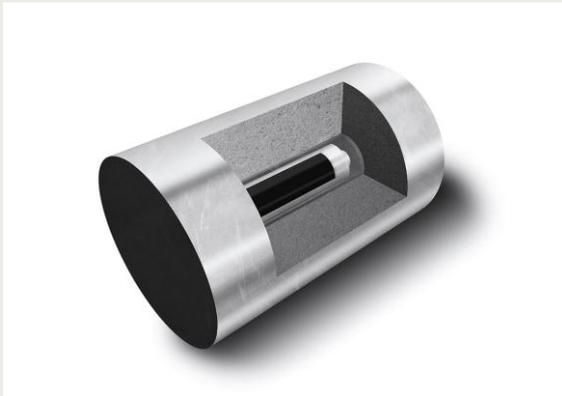
Figure 5-5 Artist impression of OPERA supercontainer for heat-generating HLW.
